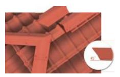
• Cut the SLIM CAP with an angle of 45° and fix it. The ridge piece has to overlap the hips.
