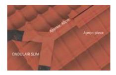
• Secure the watertightness of the detail by applying ONDULAIR SLIM.
