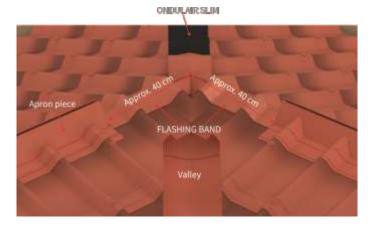
• Install APRON PIECE at ridge, ONDULAIR SLIM at hip, and a strip of FLASHING BAND (W 15cm) or ONDULAIR SLIM at meeting point.
