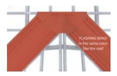
Prepare and cut the appropriate shape and surface of FLASHING BAND membrane, and apply it with care to ensure secured waterproofing.
