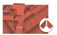
Apply module consisting of 2 SLIM CAPS portions (to be fixed together using or ONDULAIR SLIM), cutting them at the right angle in accordance with the slope of the roof
